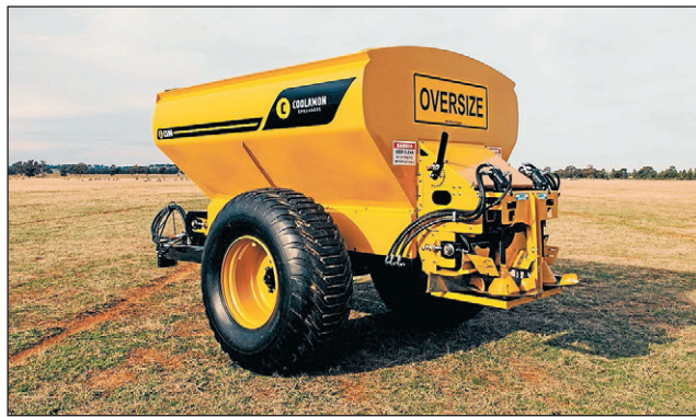
The Coolamon CS range of spreaders is the only one on the market with a one metre cleated belt and variable sized cones. Photo supplied.
